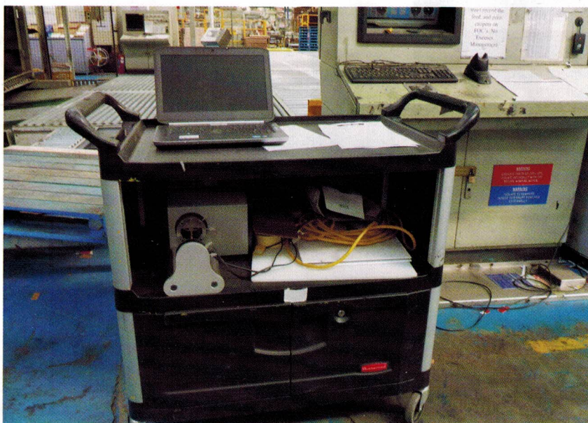
THIS DST AT AN AUSTRALASIAN BOX PLANT USES WI-FI TO CONNECT TO THE PLANT'S DATABASE COMPUTER SO THE INFORMATION IS AVAILABLE IMMEDIATELY.
